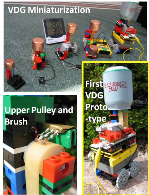
Fig. 2 Programmable robotic VDG generator; miniaturization and upper pulley.
